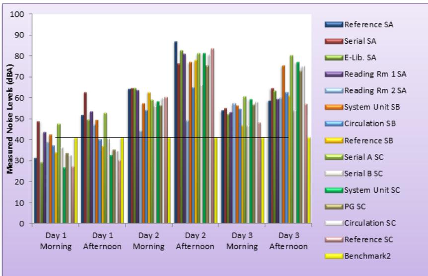
Figure 7: Benchmark on Acoustics compared with the measured noise level
