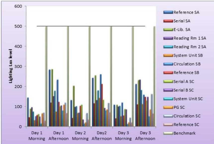
Figure 6: Lighting benchmark standard compared with the existing light lux level
