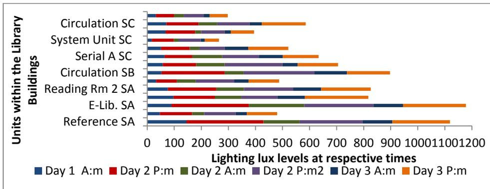
Figure 1: Collected lighting lux level of the three library buildings
