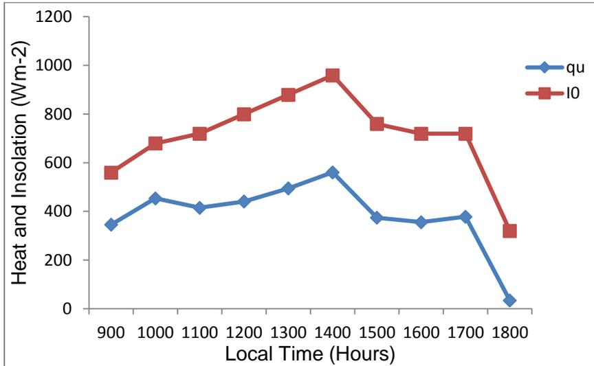
Figure 5: Heat and insolation profile showing hourly variation for 02-02-17 on no-load
