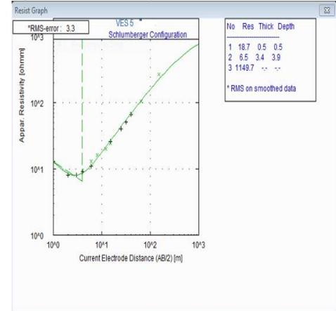
Figure 7: Resistivity curve for VES 5
