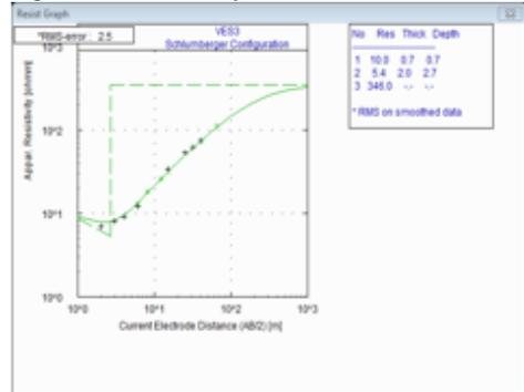
Figure 5: Resistivity curve for VES 3
