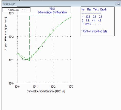
Figure 3: Resistivity curve for VES 1
