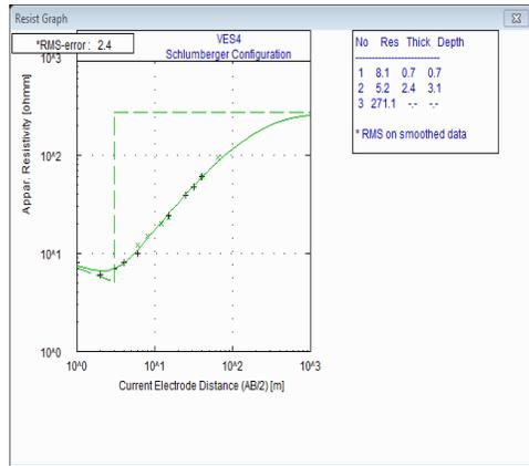
Figure 6: Resistivity curve for VES 4
