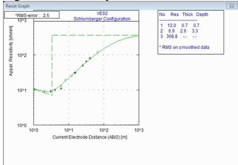
Figure 4: Resistivity curve for VES 2
